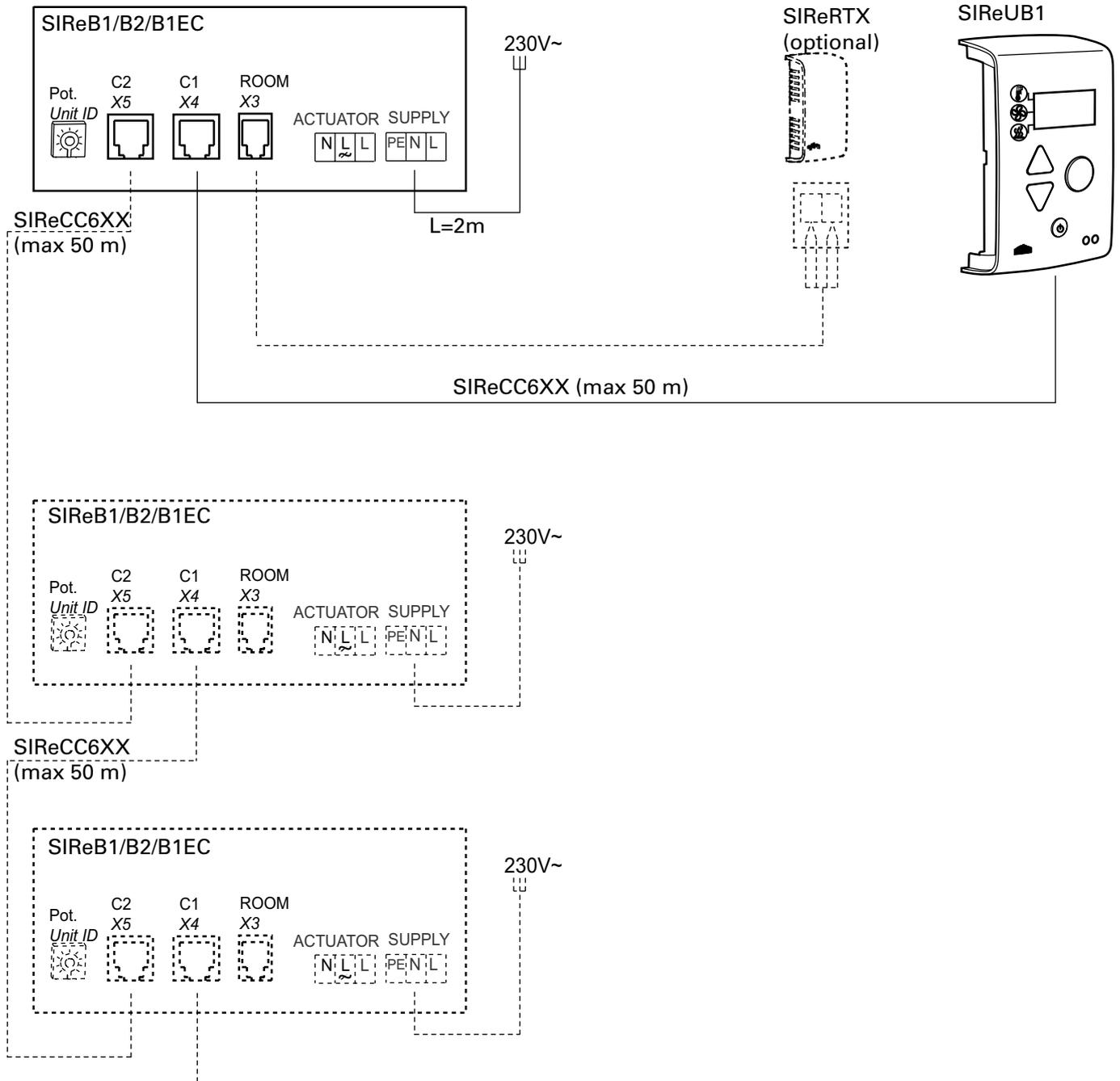
Wiring diagrams for SIReAC Competent and SIReAA Advanced, see manual for SIRe.
